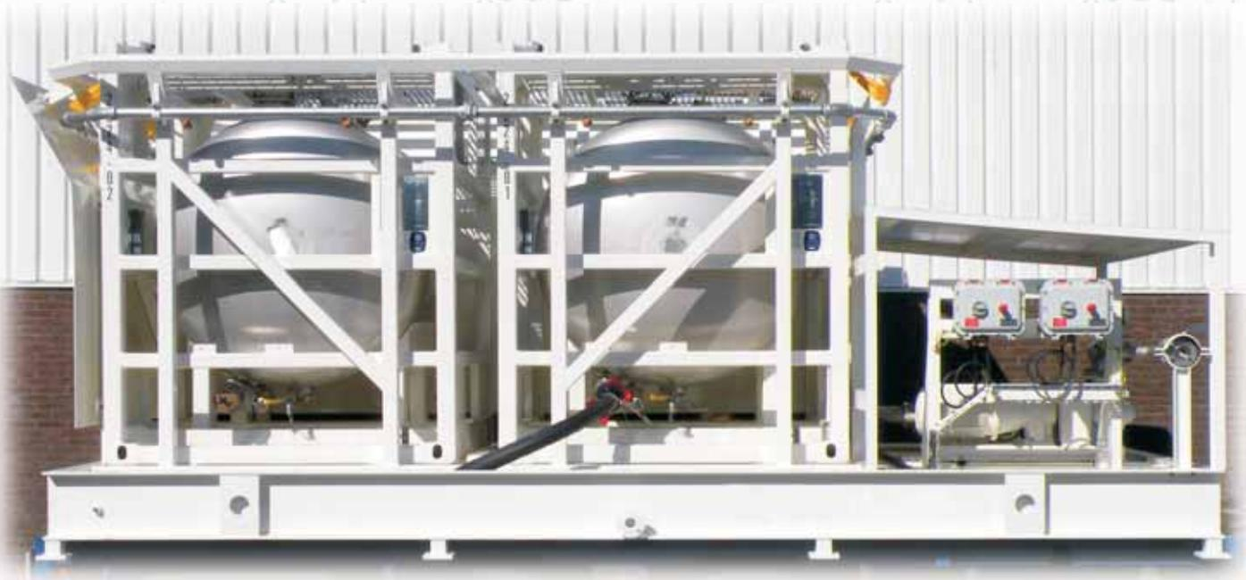
The skid will be equipped with a drip tray over complete area, 4 lifting lugs, buffer frame and deluge line.
